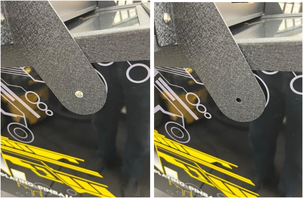
Carefully remove the head and rest somewhere safe. Two people are required to remove the head.
