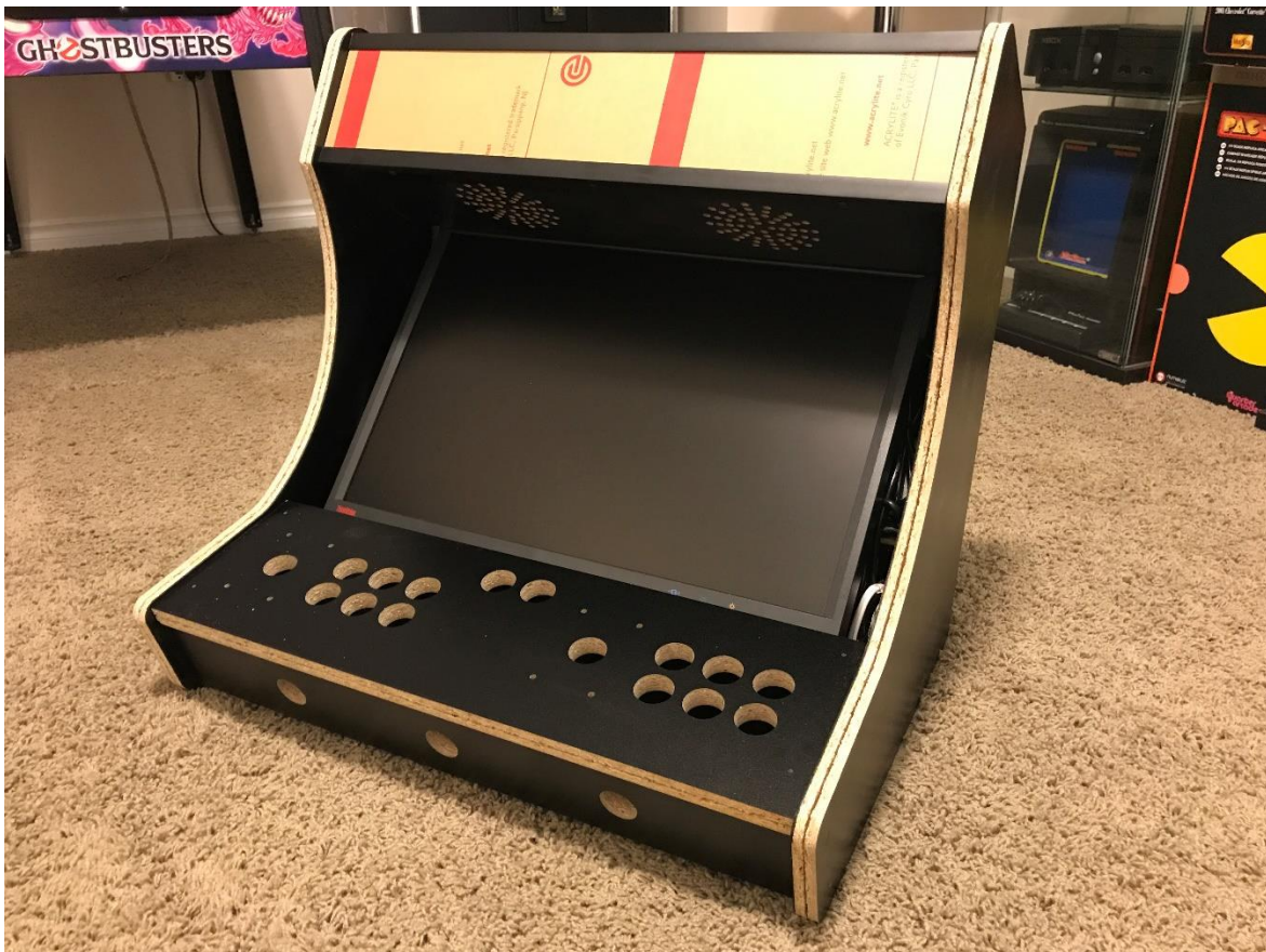
Below is an assembled cabinet with black L channel to hold Maquee plexiglass in place. I have installed a 22" LCD. Leave room for bezel and LCD plexiglass between speaker panel and LCD.
